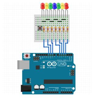
6. Add a  $470\Omega$  resistor from the pushbutton to a part of the Breadboard with no wire.
