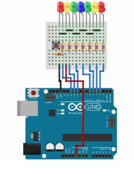
7. Connect Pin 2 of the Arduino to the left side of the pushbutton with a different coloured wire. Must be in Pin 2 for the Pushbutton.
